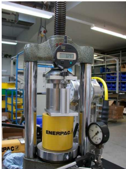
Hydraulic piston and pellet mold with digital length indicator
